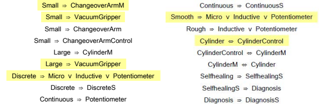
Figure 4: Cross-tree constraints based on the mapping matrix [11, 19]. Highlighted constraints are redundant.
